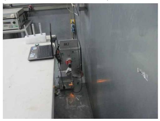
Description: Front View of Conducted Emission Test Setup
